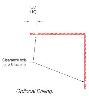
• Standard spacing: 3" (76) from each end and spaced evenly not to exceed 36" (914) oc
