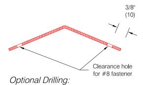
• Standard spacing: 3" (76) from each end and spaced evenly not to exceed 36" (914) oc
