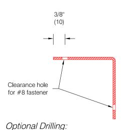
• Standard spacing: 3" (76) from each end and spaced evenly not to exceed 36" (914) oc
