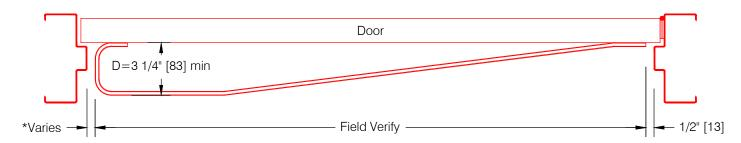
\*Clearance must increase to accommodate door swing with increase in depth (D). Standard clearance of 1/2" is adequate for standard 3 1/4" (83) depth (shown), to 4" (102) depth.
